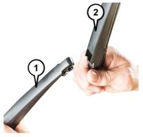
Wiper Blade Removed From Wiper Arm
