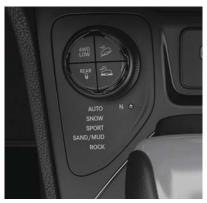
2-Speed 4x4 Switch (with Rear Lock)
