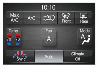
Uconnect 3 With 5-inch Display With Automatic Temperature Controls (If Equipped)
