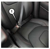
**Inserting Latch Plate Into Buckle**
