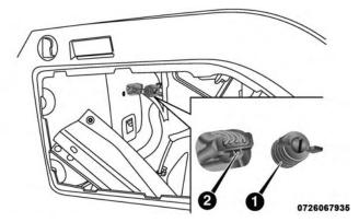
Rear Lamp Fastener and Electrical Connector
