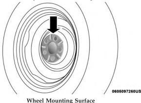
Tighten the wheel bolts in a star pattern until each bolt has been tightened twice. Ensure that the socket is fully engaged on the lug nut/bolt.
