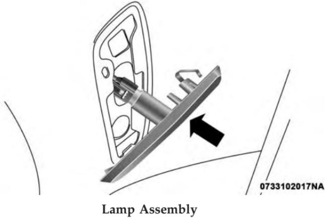
3. Remove the electrical connector by pushing the tab then disconnect the electrical connector.
