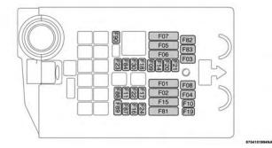
**Engine Compartment Fuse Cavities**
