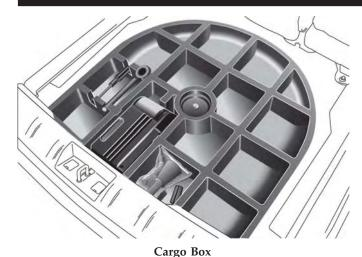
**NOTE:** The cargo box is sized for a maximum capacity of distributed weight equal to 242 lbs (110 kg).
