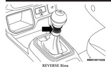
To engage REVERSE gear from the NEUTRAL position, lift the REVERSE ring, located below the knob and simultaneously move the lever to the left and then forward.
