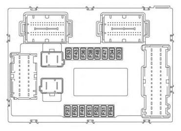
**Body Controller Fuse Cavities**
