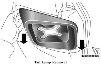
6. Unscrew the screws and remove the rear tail lamp holder.
