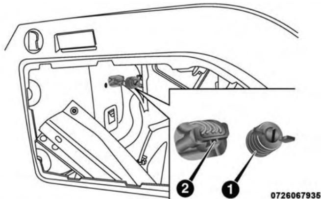
Rear Lamp Fastener and Electrical Connector
