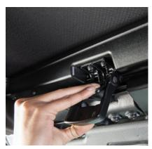
Squeeze Latch Plate And Pull Handle Upward
