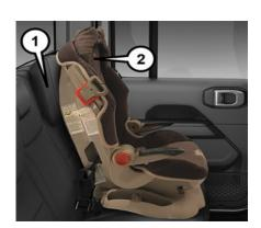
**Car Seat With Head Restraint Folded**
