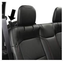
**Rear Head Restraint Folding Strap Location**
