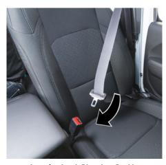
**Inserting Latch Plate Into Buckle**
