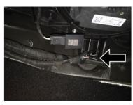
Auxiliary Switch Connections – Under Instrument Panel
