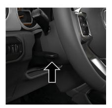
Tilt/Telescoping Steering Column Lever
