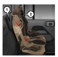
**Car Seat With Head Restraint Folded**
