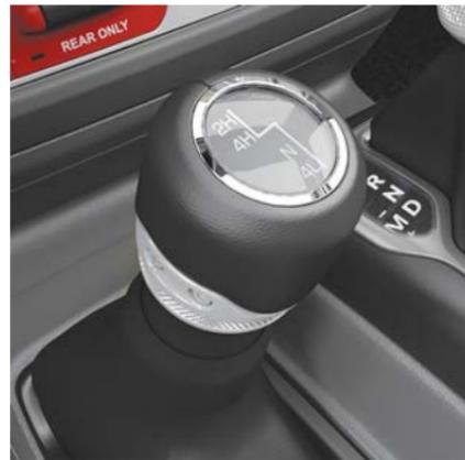
**Four Position Four-Wheel Drive Gear Selector**
