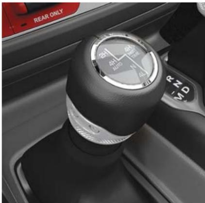
**Five Position Four-Wheel Drive Gear Selector**
