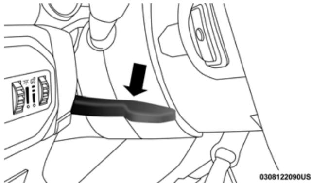
Tilt/Telescoping Steering Column Lever
