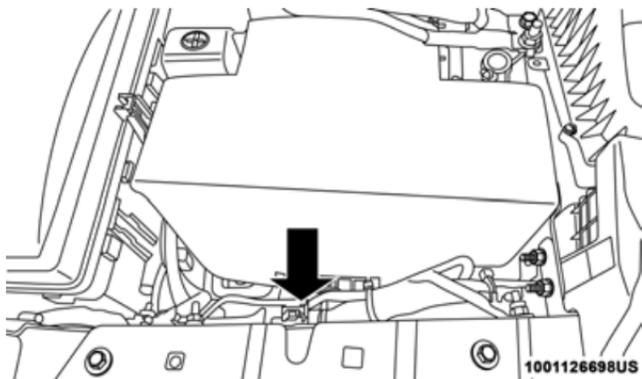
**Auxiliary Switch Connections – Under Hood**
