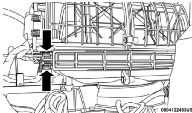
**Air Filter Retaining Tabs**
