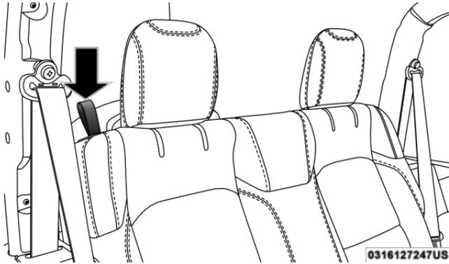
**Rear Head Restraint Folding Strap Location**
