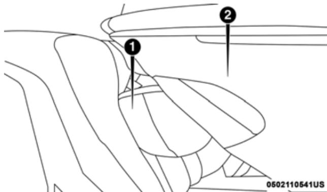
**Car Seat With Head Restraint Folded**
