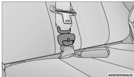
Inserting Mini-Latch Plate Into Mini-Buckle
