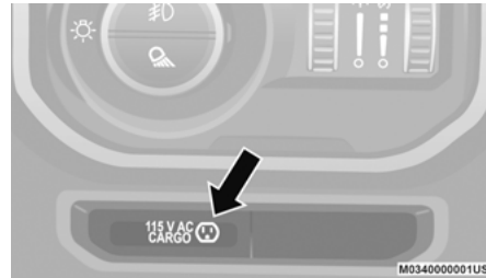
Power Inverter Switch (If Equipped)
