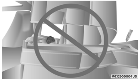
Incorrect Placement Of Wire Harness
