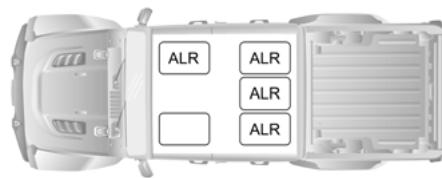
ALR — Switchable Automatic Locking Retractor
