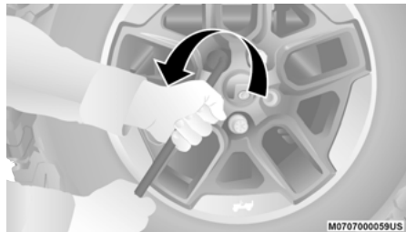
Removing The Spare Tire
