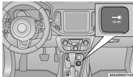
Front Power Outlet
