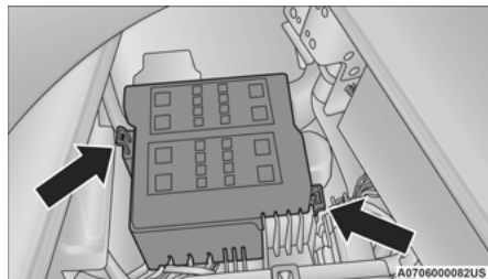
Rear Cargo Fuse Panel Cover
