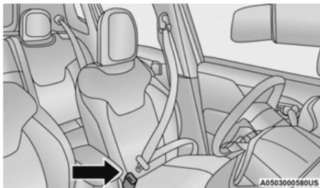
**Inserting Latch Plate Into Buckle**
