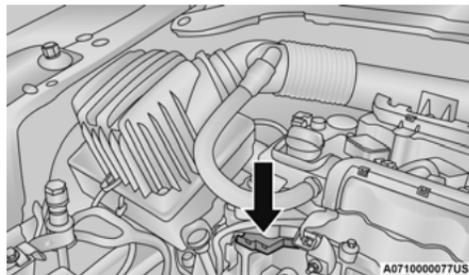
**Suitable Engine Ground (Example Engine Shown)**
