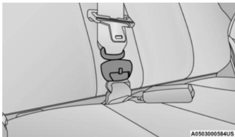
**Inserting Mini-Latch Plate Into Mini-Buckle**
