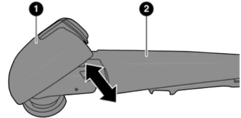
**Wiper Pivot Cap In Unlocked Position**
