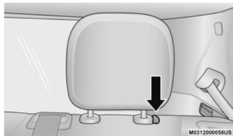
**Outboard Head Restraint Adjustment Button**
