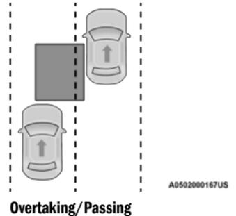
The BSM system is designed not to issue an alert on stationary objects such as guardrails, posts, walls, foliage, berms, etc. However, occasionally the system may alert on such objects. This is normal operation and your vehicle does not require service.
