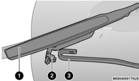
**Removing Wiper From Wiper Arm**
