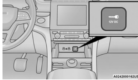
Front Power Outlet
