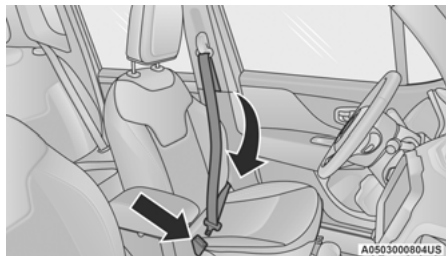
Pulling Out The Latch Plate
