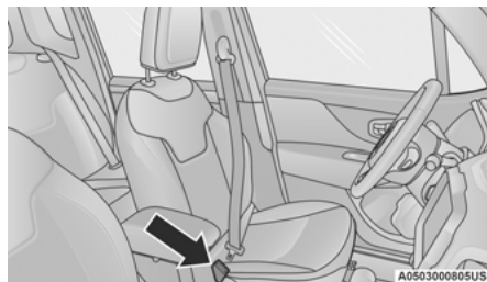
Inserting Latch Plate Into Buckle
