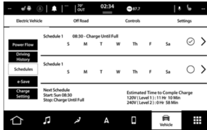
Charging Schedules Screen
