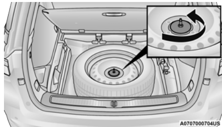
Removing The Spare Tire Fastener
