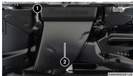
First Water Separation Chamber
