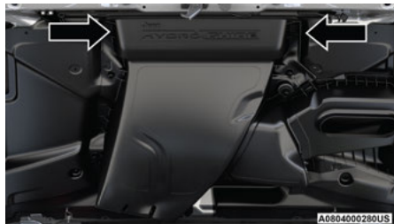
First Water Chamber Removal
