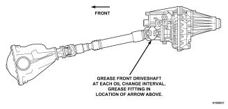
Front Driveshaft Grease Fitting
