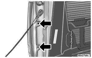
2. Pull the housing straight out from the body, with a quick motion, to separate the housing from the body. If not pulled straight, locators may be damaged.
