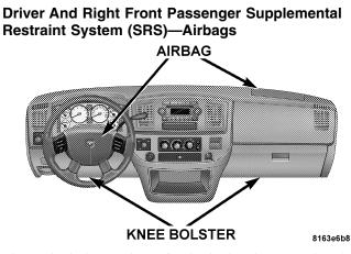
This vehicle has airbags for both the driver and right front passenger as a supplement to the seat belt restraint systems. The driver's front airbag is mounted in the steering wheel. The passenger front airbag is mounted in the instrument panel, above the glove compartment. The words SRS/AIRBAG are embossed on the airbag covers.
