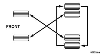
**NOTE:** On Canadian vehicles only, if your Ram truck is equipped with All-Season type tires on the front and ON/OFF Road type tires mounted on the rear, do not use a front to back rotation pattern. Instead, rotate your tires side to side at the recommended intervals.
