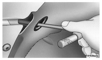
**Rear Headlight Housing Nut Access** 4. Pull the housing out from the fender to allow room to disconnect the electrical connectors. **NOTE:** For easier removal, pull the headlight assembly straight forward, applying the greatest amount of force to the outer edge of the headlight assembly.
