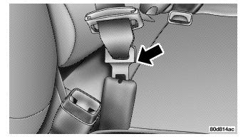
**Inserting Latch Plate**
