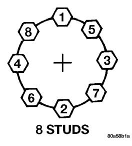
1. Tighten the wheel nuts in the numbered sequence to a snug fit.
