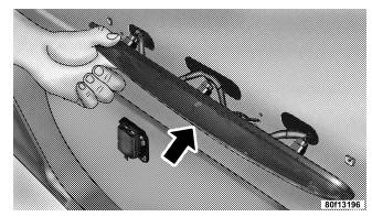
2. Turn socket <sup>1</sup>/<sub>4</sub> turn counterclockwise to access the bulb.
