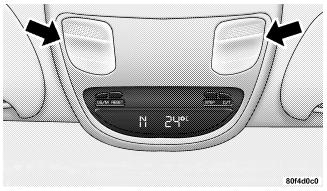
This overhead console allows you to choose between a compass/temperature display and one of four trip conditions being monitored.
