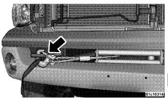
20. Disconnect the remote control. Disconnect the remote control cord from the control box and store in a clean and dry place. Winching operations are now complete. Put the cap on the solenoid plug-in.
