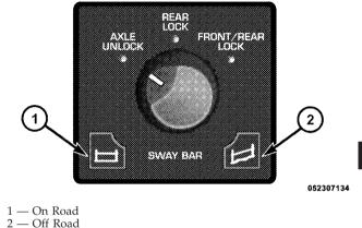
The switch has two positions; On-Road and Off-Road. The system is normally in the On-Road mode, indicated by a solid green light. The stabilizer/sway bar should remain in the On-Road mode during normal driving conditions.
