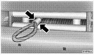
1. Inspect the winch, winch mount, and wire rope for damage. Do not use the winch if the mount is loose or rope shows excessive wear or damage.
