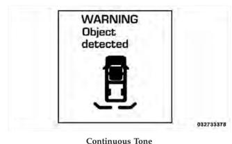
The vehicle is close to the obstacle when the EVIC display shows one flashing arc and sounds a continuous tone. The following chart shows the warning alert operation when the system is detecting an obstacle:
