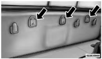
Mega Cab<sup>®</sup> Tether Strap Mounting 3. Install the child restraint and remove the slack in the tether strap according to the manufacturer's instructions.
