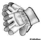
**Gloves:** Wire rope, through use, will develop "barbs" which can slice skin. It is extremely important to wear protective gloves while operating the winch or handling the wire rope. Avoid loose fitting clothes or anything that could become entangled in the wire rope and other moving parts.
