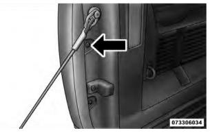
2. Pull the outboard side of the lamp rearward far enough to unsnap the two receptacles on the outboard side of the lamp housing from the two plastic snap post retainers in the outer box side panel.
