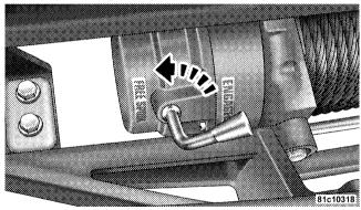
4. Free the winch hook and attach the hook strap. Free the winch hook from its anchor point. Attach the hook strap to the hook (if not attached).
