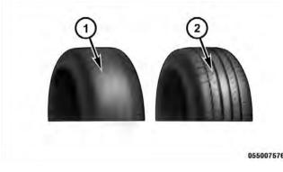
1 — Worn Tire 2 — New Tire These indicators are molded into the bottom of the tread grooves. They will appear as bands when the tread depth becomes 1/16 in (2 mm). When the tread is worn to the tread wear indicators, the tire should be replaced.
