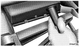
10. Put wire rope under tension. Using the remote control switch, slowly wind the wire rope until no slack remains. Once the wire rope is under tension, stand well clear of it and never step over it.
