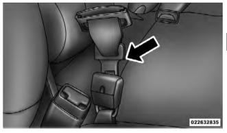
**Inserting Latch Plate**
