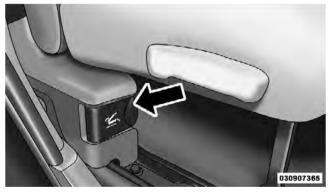
**Handle** 2. Fold the seatback down and push the seat forward.
