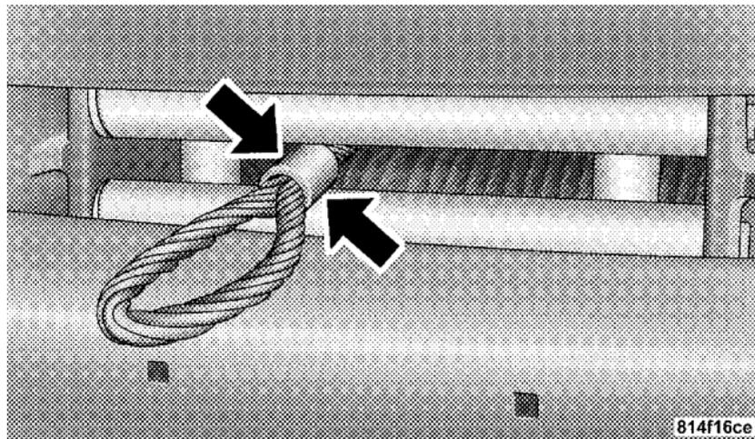
1. Inspect the winch, winch mount, and wire rope for damage. Do not use the winch if the mount is loose or rope shows excessive wear or damage.
