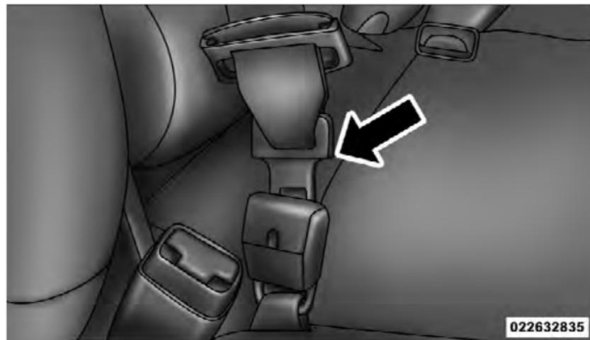
Inserting Latch Plate
