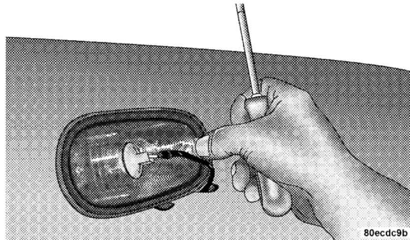
3. Pull the bulb straight from it's socket and replace.
