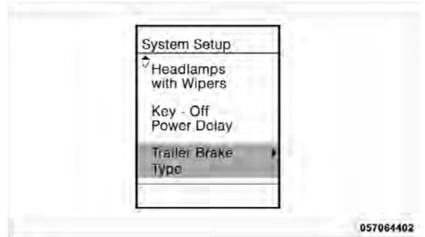
6. Press the SELECT button and then press the UP or DOWN buttons until the proper Trailer Brake Type appears on the screen.
