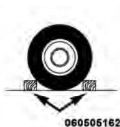
6. Block both the front and rear of the wheel diagonally opposite the jacking position. For example, if the right front wheel is being changed, block the left rear wheel.
