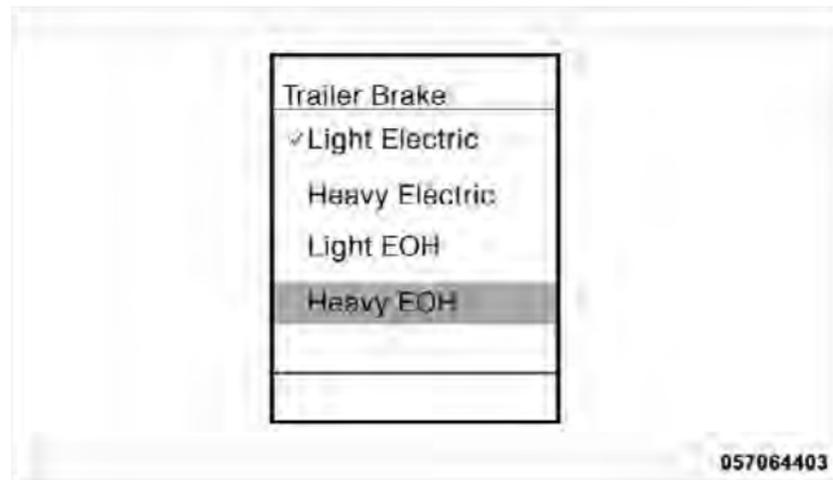
**NOTE: 1500 Models Only** – Light Electric and Heavy Electric will only be available due to the tow capacities of the vehicle.
