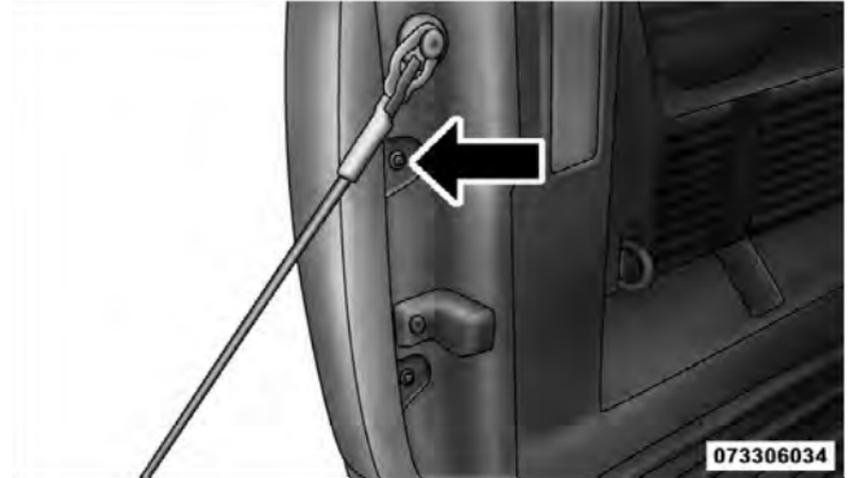
2. Pull the outboard side of the lamp rearward far enough to unsnap the two receptacles on the outboard side of the lamp housing from the two plastic snap post retainers in the outer box side panel.
