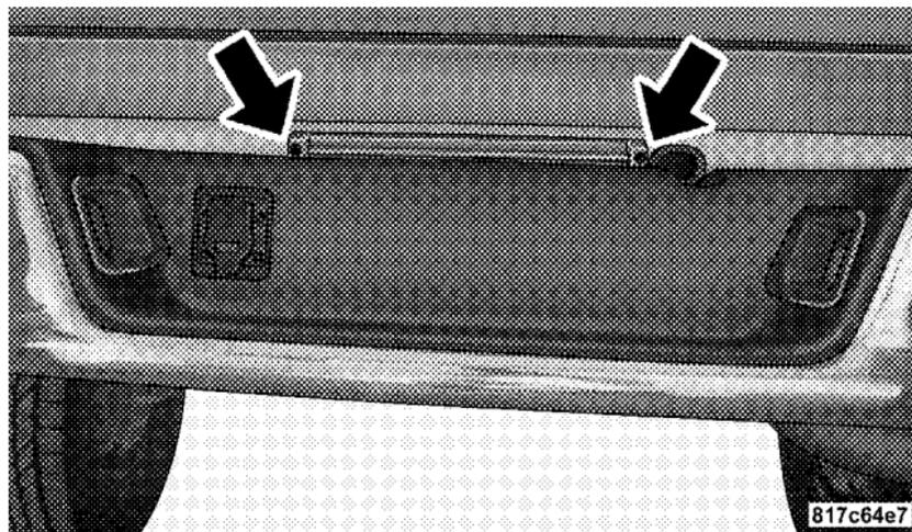
2. Turn the socket  $\frac{1}{4}$  turn counterclockwise to access the bulb.
