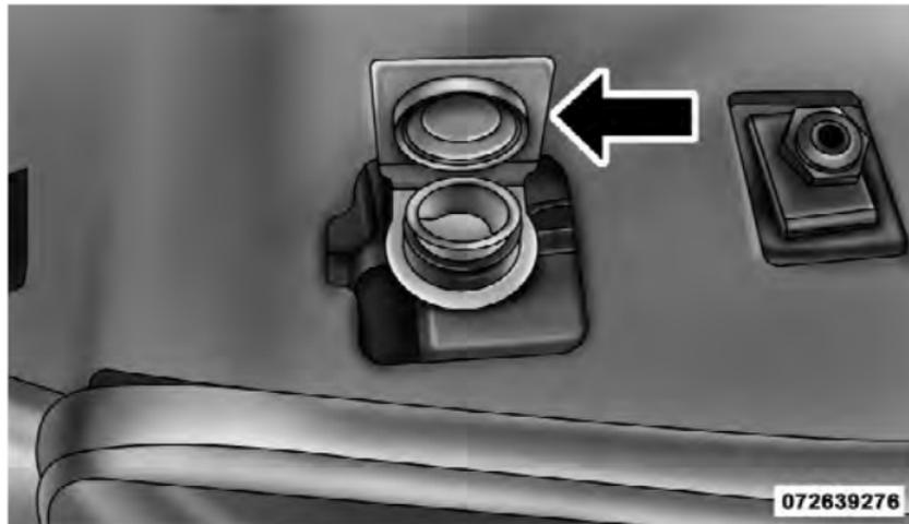
2. Lift and remove the plastic dipstick from the reservoir neck.
