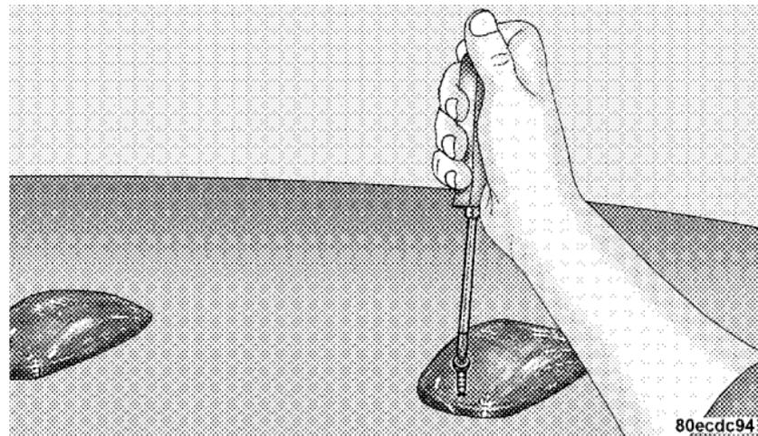
2. Rotate the socket  $\frac{1}{4}$  turn and pull it from the lamp assembly.
