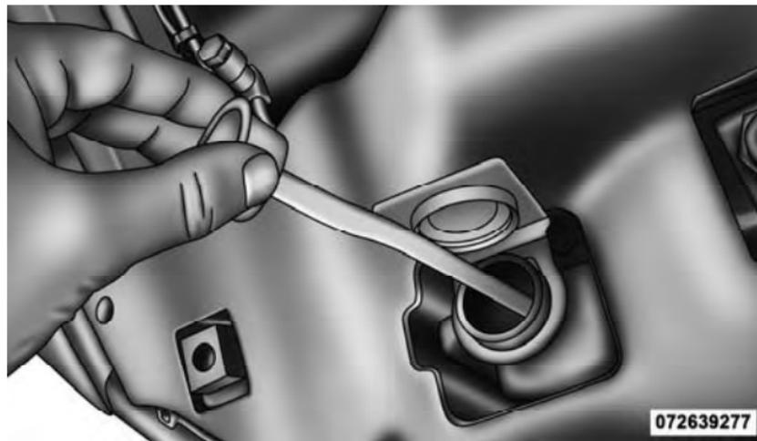
3. Check the coolant level on the dipstick.
