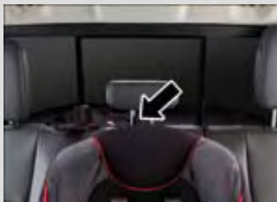
Tether Strap Through Center Tether Strap Loop
