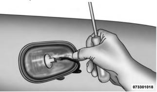
Removing Bulb Socket From Clearance Lamp
