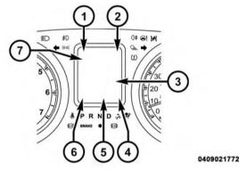
The EVIC displays are located in the center portion of the cluster and consists of seven sections:
