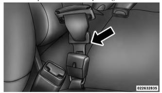
**Inserting Latch Plate**
