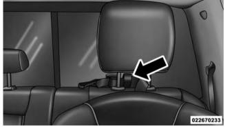
Tether Strap Through Outboard Tether Strap Loop
