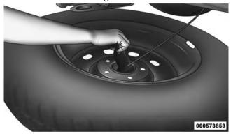
Pulling The Retainer Through The Center Of The Wheel **NOTE:** The winch mechanism is designed for use with the jack extension tube only. Use of an air wrench or other power tools is not recommended and can damage the winch.
