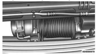
Wire Neatly Wound Around The Spooling Drum
