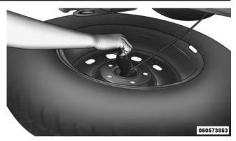
Reinstalling The Retainer
