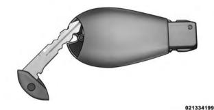
Separating Ignition Node Module (IGNM) Transmitter
