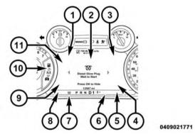
The EVIC displays are located in the center portion of the cluster and consists of eight sections:
