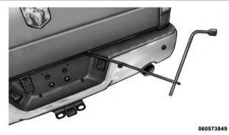
Wheel Wrench And Jack Extension Tube Assembled
