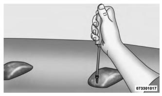
Removing Rear Screw From Clearance Lamp
