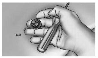
Removing The Bulb From The Bulb Socket
