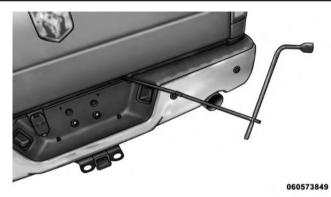
Wheel Wrench And Jack Extension Tube Assembled
