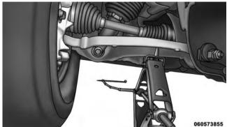
**4X4 Front Jacking Location** 4x2 and 4x4 Rear Jacking Location
