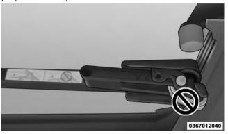
Improper Clamp Wire Released Position
