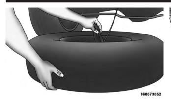
Pulling The Retainer Through The Center Of The Wheel Wrench And Jack Extension Tube Assembled And And Positioning It
