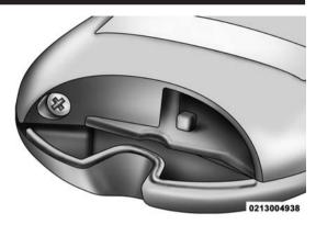
Remove Screw From Transmitter Case
