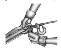
8. Lock the clutch. Lock the winch drum by rotating the clutch lever on the winch to engage.
