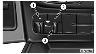
**Integrated Trailer Brake Module (ITBM)**
