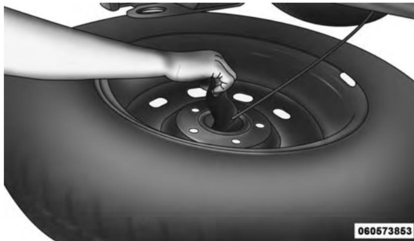
Reinstalling The Retainer
