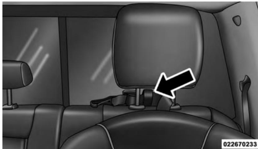
**Tether Strap Through Outboard Tether Strap Loop**
