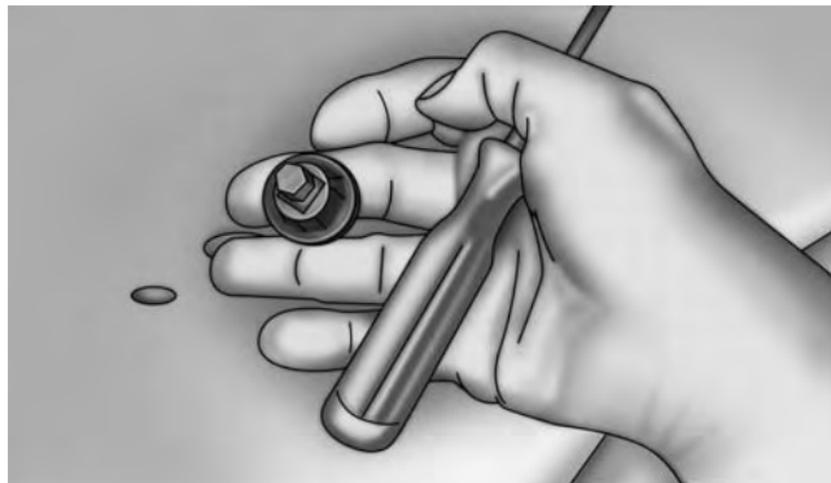
**Removing The Bulb From The Bulb Socket
