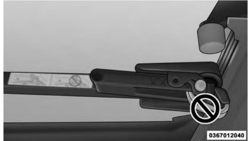
Improper Clamp Position
