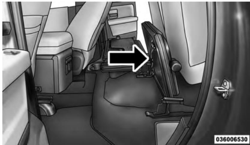
**Load Floor Securing Straps**
