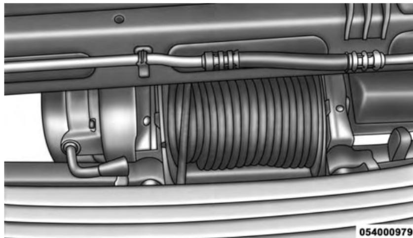
Wire Neatly Wound Around The Spooling Drum
