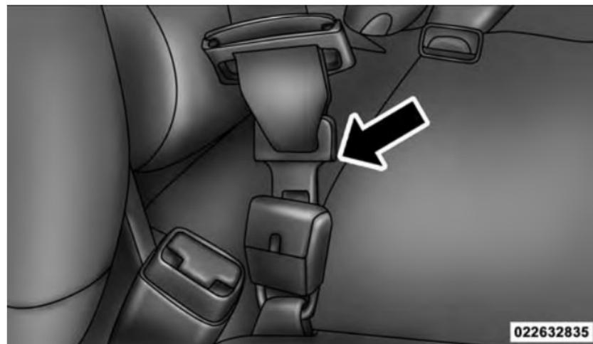
Inserting Latch Plate
