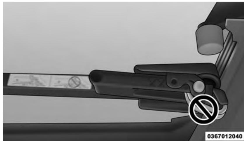
**Improper Clamp Wire Released Position**
