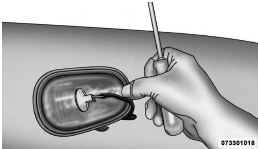
**Removing Bulb Socket From Clearance Lamp**
