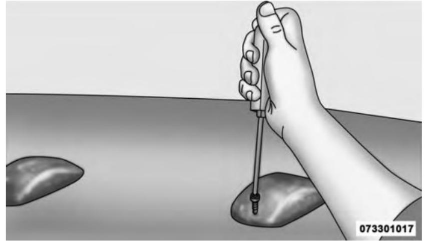
Removing Rear Screw From Clearance Lamp
