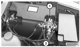
Battery (Diesel Model Shown)
