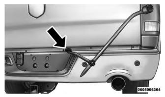
Inserting The Jack Extension Tube Into The Access Hole
