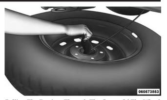
**Pulling The Retainer Through The Center Of The Wheel NOTE:** The winch mechanism is designed for use with the jack extension tube only. Use of an air wrench or other power tools is not recommended and can damage the winch.
