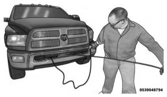
Pulling Wire Rope Under Tension
