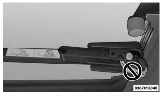
Improper Clamp Wire Released Position
