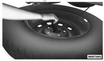
**Reinstalling The Retainer**
