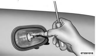
Removing Bulb Socket From Clearance Lamp
