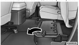
**Unfolding The Load Floor**
