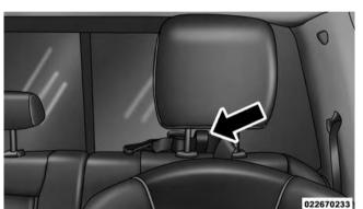
Tether Strap Through Outboard Tether Strap Loop
