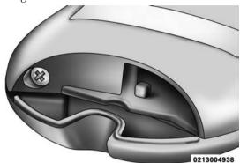
Remove Screw From Transmitter Case
