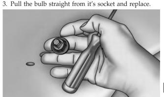
Removing The Bulb From The Bulb Socket
