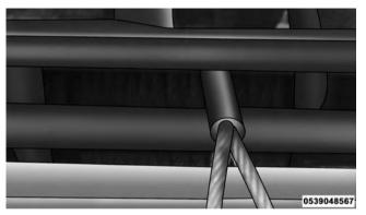
Wire Neatly Wound Around The Spooling Drum
