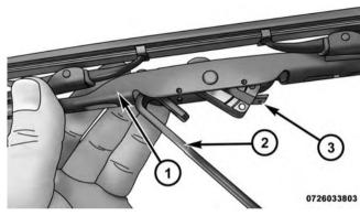
Wiper Blade Removed From Wiper Arm
