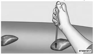
Removing Rear Screw From Clearance Lamp
