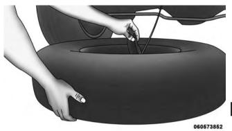
Gaining Access To The Retainer 5. Pull the retainer through the center of the wheel.
