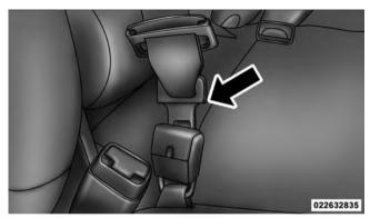
**Inserting Latch Plate**
