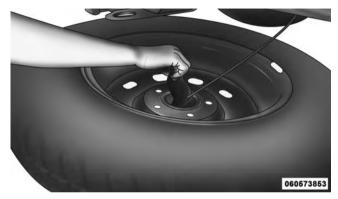
Reinstalling The Retainer
