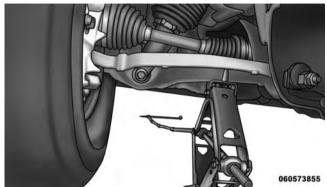
**4X4 Front Jacking Location** 4x2 and 4x4 Rear Jacking Location
