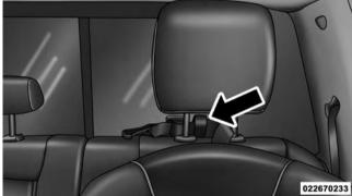
Tether Strap Through Outboard Tether Strap Loop
