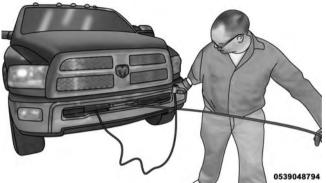
**Pulling Wire Rope Under Tension**
