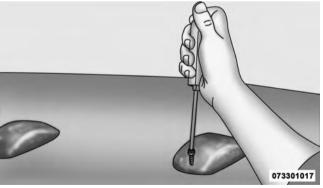
Removing Rear Screw From Clearance Lamp
