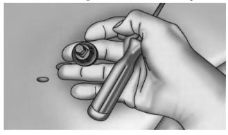
Removing The Bulb From The Bulb Socket
