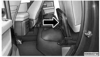
Load Floor Securing Straps/Crew Cab
