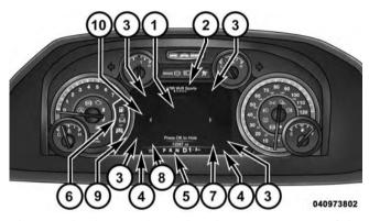
The DID displays are located in the center portion of the cluster and consists of eight sections:
