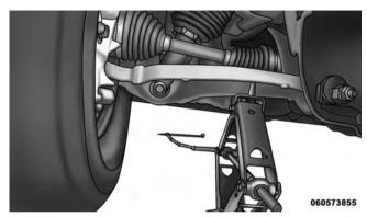
4X4 Front Jacking Location 4x2 and 4x4 Rear Jacking Location
