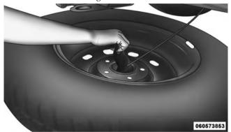
Reinstalling The Retainer
