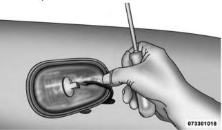
Removing Bulb Socket From Clearance Lamp
