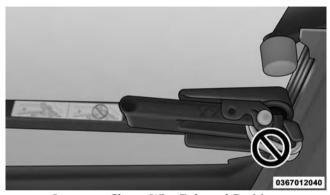
Improper Clamp Wire Released Position
