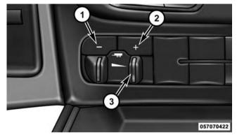
**Integrated Trailer Brake Module (ITBM)**
