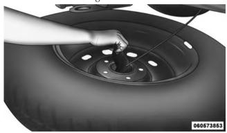
**Reinstalling The Retainer**
