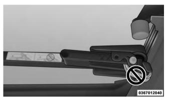
Improper Clamp Position
