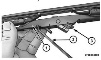
Wiper Blade Removed From Wiper Arm
