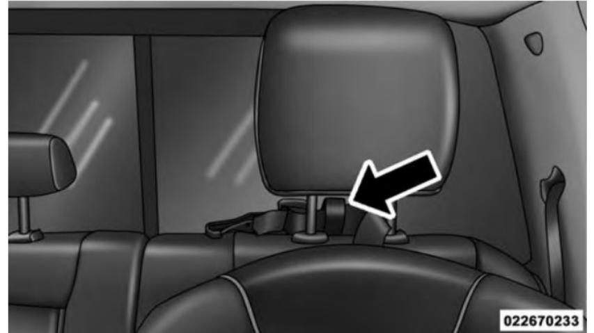
**Tether Strap Through Outboard Tether Strap Loop**
