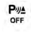
When the ParkSense switch is pushed to disable the system, the instrument cluster will display the “PARKSENSE OFF” message for approximately five seconds. Refer to “Electronic Vehicle Information Center (EVIC) or Driver Information Display (DID)” in “Understanding Your Instrument Panel” for further information. When the gear selector is moved to REVERSE and the system is disabled, the EVIC/DID will display the “PARKSENSE OFF” message for as long as the vehicle is in REVERSE.
