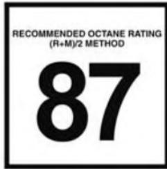
This engine is designed to meet all emissions regulations and provide optimum fuel economy and performance when using high quality unleaded "Regular" gasoline having a posted octane number of 87 as specified by the (R+M)/2 method. The use of
