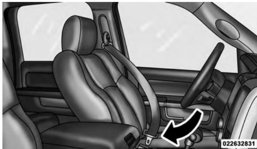
**Inserting Latch Plate Into Buckle**
