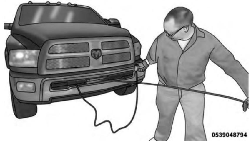
**Pulling Wire Rope Under Tension**
