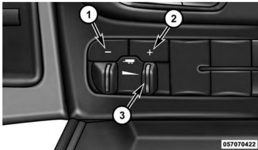
Integrated Trailer Brake Module (ITBM)
