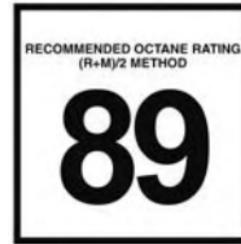
This engines is designed to meet all emissions regulations and provide satisfactory fuel economy and performance when using high quality unleaded gasoline having a posted octane number range of 87 to 89 as specified by the (R+M)/2 method. The
