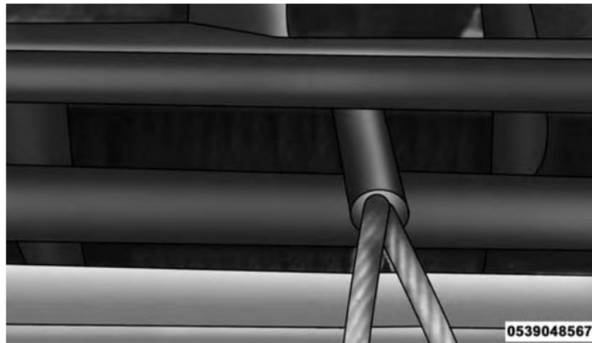
Wire Neatly Wound Around The Spooling Drum
