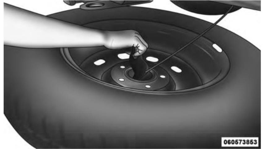
Reinstalling The Retainer
