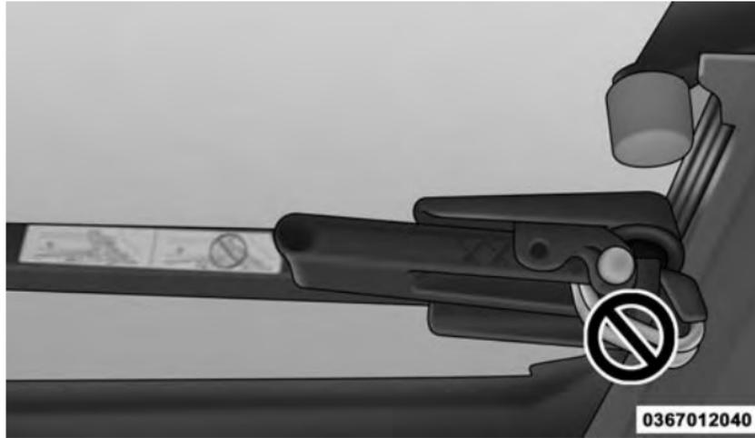
Improper Clamp Wire Released Position
