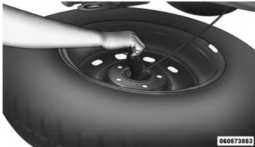
Reinstalling The Retainer
