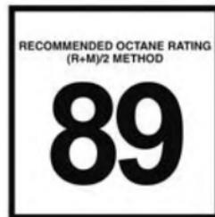
This engine is designed to meet all emissions regulations and provide satisfactory fuel economy and performance when using high quality unleaded gasoline having a posted octane number range of 87 to 89 as specified by the (R+M)/2 method. The
