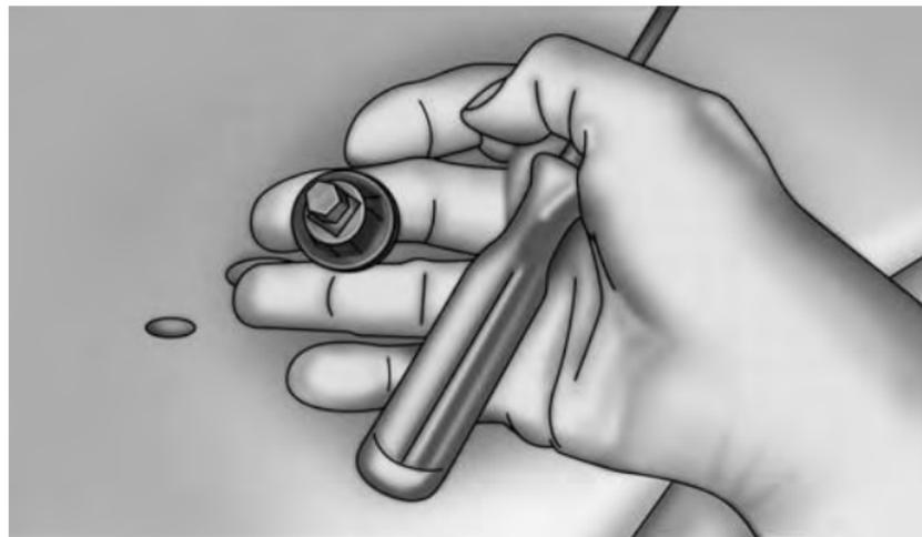
Removing The Bulb From The Bulb Socket
