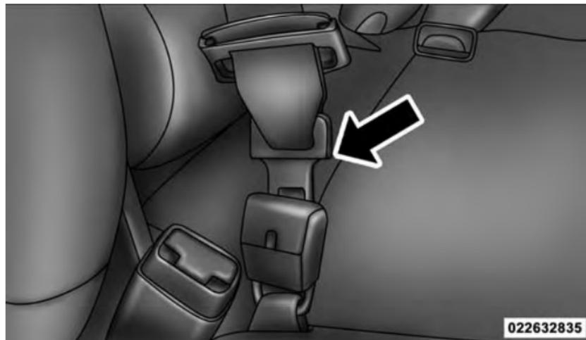
**Inserting Latch Plate**
