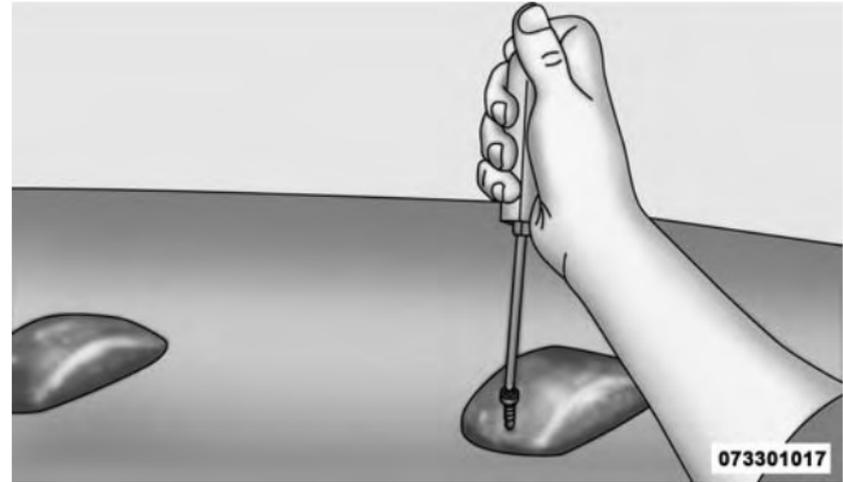
Removing Rear Screw From Clearance Lamp
