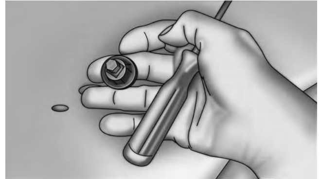
Removing The Bulb From The Bulb Socket
