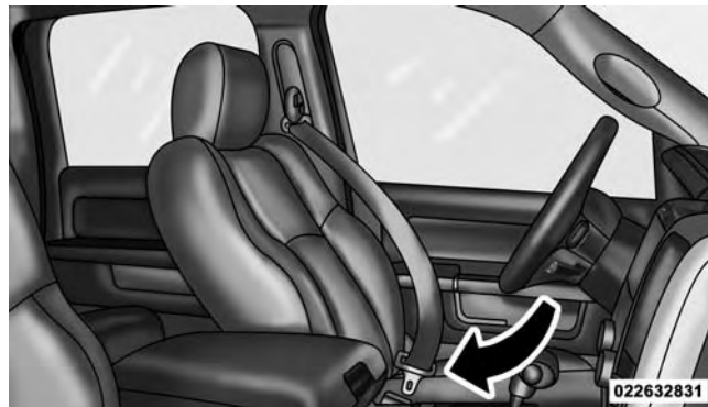
Inserting Latch Plate Into Buckle
