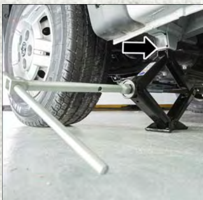
Front Jacking Location
