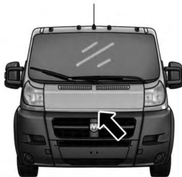
Hood Safety Latch Lever Location
