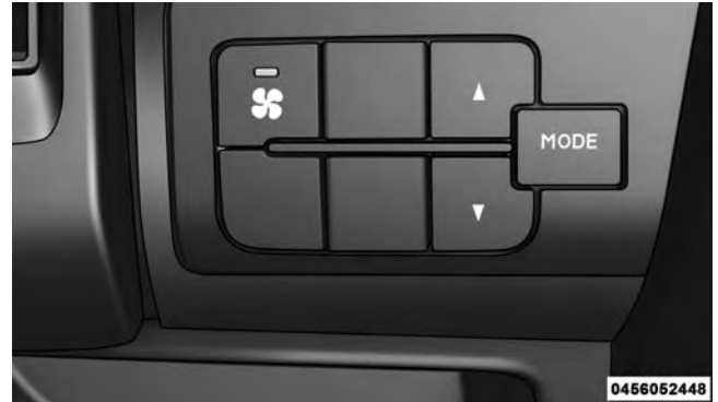
Additional Rear Climate Control Switch
