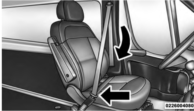
Inserting Latch Plate Into Buckle
