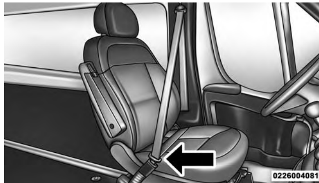
Pulling Out The Latch Plate
