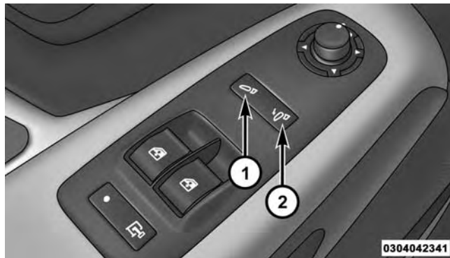
Power Folding Mirror Switch
