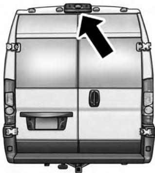
Rear Back Up Camera Location
