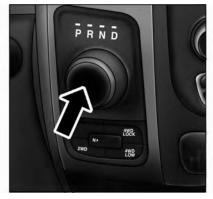
**Electronic Transmission Gear Selector**
