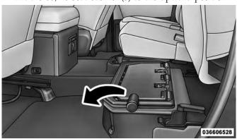
**Unfolding The Load Floor**
