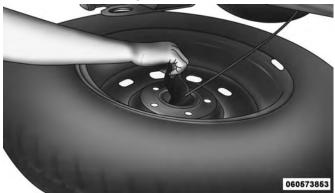
Reinstalling The Retainer
