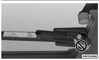
Improper Clamp Wire Released Position
