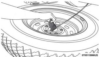
Pulling The Retainer Through The Center Of The Wheel **NOTE:** The winch mechanism is designed for use with the extension tubes only. Use of an air wrench or other power tools is not recommended and can damage the winch.
