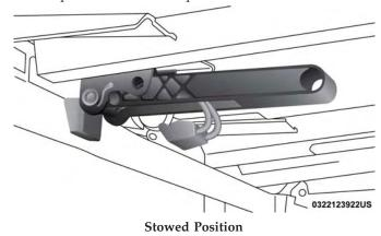
3. Push clamp wires up and under the flange of box (or flange of Ram Box rail, if equipped) to the semi clamped position.
