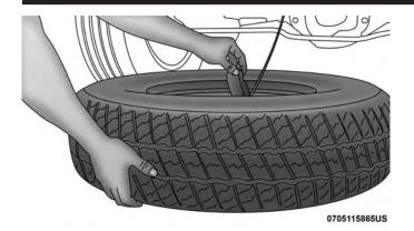
Gaining Access To The Retainer 5. Pull the retainer through the center of the wheel.
