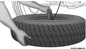
Pushing The Retainer Through The Center Of The Wheel
