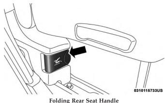
2. Fold the seatback down and push the seat forward.
