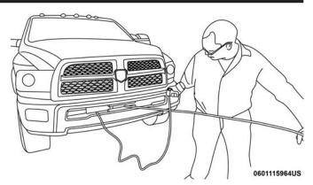
**Pulling Wire Rope Under Tension**
