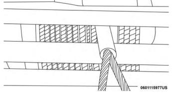
Wire Neatly Wound Around The Spooling Drum
