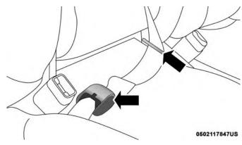
Mini-Latch And Mini-Buckle Connected
