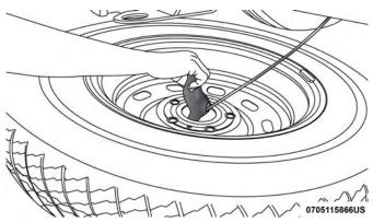
Reinstalling The Retainer
