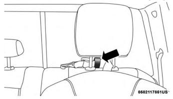
Tether Strap Through Outboard Tether Strap Loop
