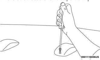
Removing Rear Screw From Clearance Lamp
