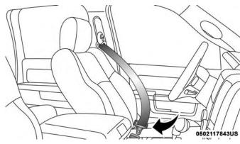
**Inserting Latch Plate Into Buckle**
