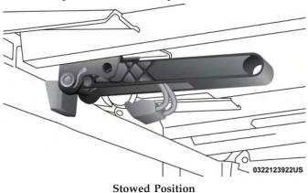
9. Push clamp wires up and under the flange of box (or flange of Ram Box rail, if equipped) to the semi clamped position.
