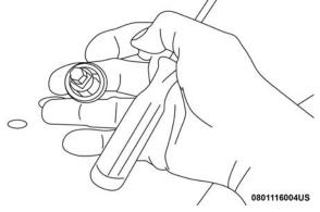
Removing The Bulb From The Bulb Socket
