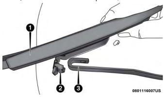
Removing Wiper From Wiper Arm
