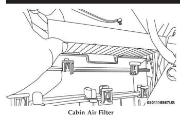
7. Install the cabin air filter with the arrow on the filter pointing toward the floor. When installing the filter cover, press on each end until you hear an audible click.
