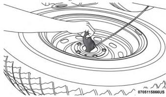
Reinstalling The Retainer
