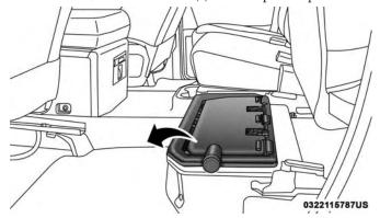
**Unfolding The Load Floor**
