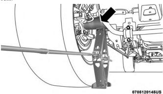
**Rear Jacking Location**Connect the extension tubes and lug wrench.
