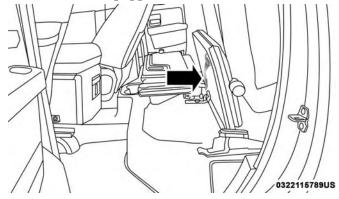
Load Floor Securing Straps/Quad Cab
