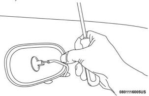
Removing Bulb Socket From Clearance Lamp
