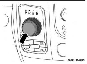
**Electronic Transmission Gear Selector**
