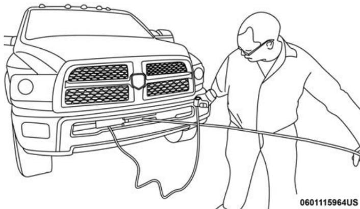
**Pulling Wire Rope Under Tension**
