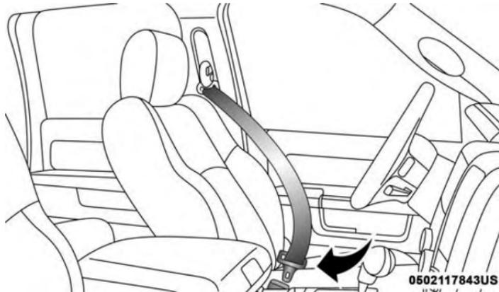
**Inserting Latch Plate Into Buckle**
