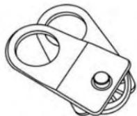
**Snatch/Block Pulley:** Used properly, the multi-purpose snatch block allows you to (1) increase the winch's pulling power; and (2) change your pulling direction without damaging the wire rope. Proper use of the snatch block is covered in "Before You Pull."
