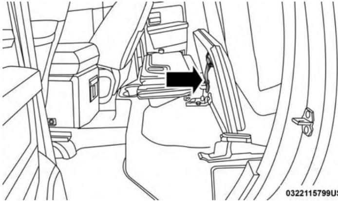
**Load Floor Securing Straps/Crew Cab**
