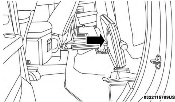
Load Floor Securing Straps/Quad Cab
