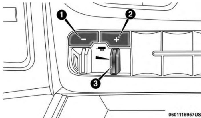
**Integrated Trailer Brake Module (ITBM)**
