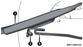
Removing Wiper From Wiper Arm
