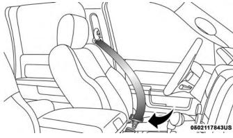
Inserting Latch Plate Into Buckle
