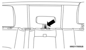
Crew Cab Center Tether Anchorage With Head Restraint
