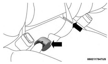
Mini-Latch And Mini-Buckle Connected
