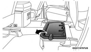
**Unfolding The Load Floor**
