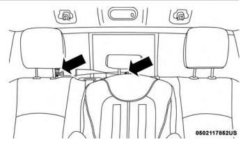
Tether Strap Through Center Tether Strap Loop And Attached To Outboard Tether Strap Loop Installing Three Child Restraints:
