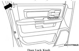
Front doors may be opened with the inside door handle without lifting the lock knob.
