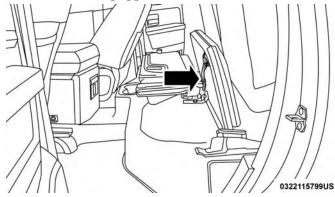
Load Floor Securing Straps/Crew Cab
