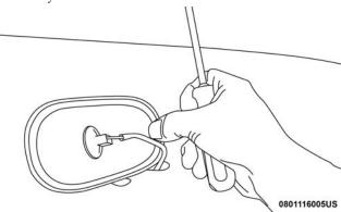
Removing Bulb Socket From Clearance Lamp
