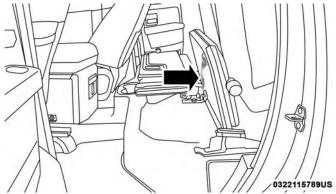
Load Floor Securing Straps/Quad Cab
