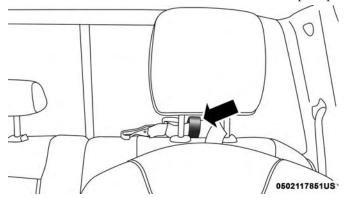
Tether Strap Through Outboard Tether Strap Loop
