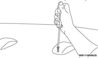
Removing Rear Screw From Clearance Lamp
