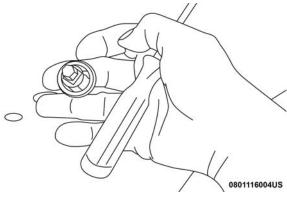
Removing The Bulb From The Bulb Socket
