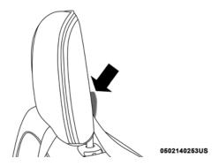
**Tether Strap Through Outboard Tether Strap Loop**
