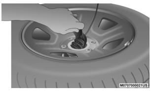
Reinstalling The Retainer
