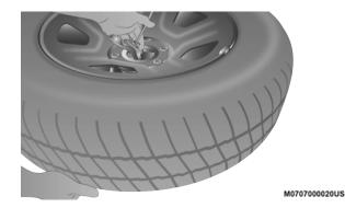
Pushing The Retainer Through The Center Of The Wheel
