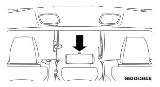
Center Tether Anchorage Over Head Rest
