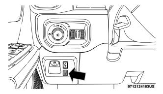
**Instrument Panel Power Inverter Switch**
