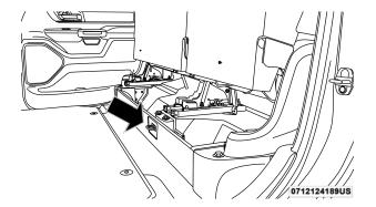
**Rotate Lock Mechanism**
