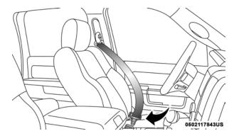
**Inserting Latch Plate Into Buckle**
