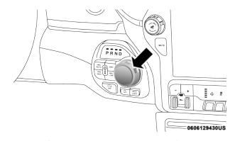
**Electronic Transmission Gear Selector**
