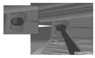
Winch Mechanism Tube
