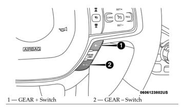
To exit ERS mode, simply push and hold the GEAR+ switch until the gear limit display disappears from the instrument cluster.
