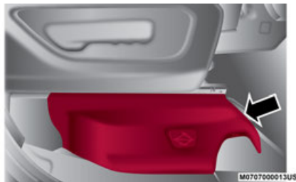
Pull Jack Access Cover From Front
