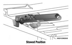
Push clamp wires up and under the flange of box (or flange of Ram Box rail, if equipped) to the semi clamped position.
