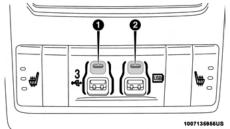
Rear Center Console Mini-USB (Type C) USB Ports
