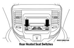
There are two heated seat switches that allow the rear passengers to operate the seats independently. You can choose from HI, MED, LO, or OFF heat settings. Amber indicator lights in each switch indicate the level of heat in use.
