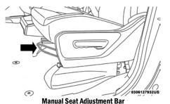
While sitting in the seat, pull up on the handle and slide the seat forward or rearward. Release the bar once you have reached the desired position. Then, using body pressure, move forward and rearward on the seat to be sure that the seat adjusters have latched.
