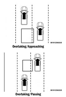
The BSM system is designed not to issue an alert on stationary objects such as guardrails, posts, walls, foliage, berms, snow banks, car washes etc. However, occasionally the system may alert on such objects. This is normal operation and your vehicle does not require service.
