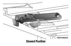
8. Clip both stowage straps to prevent the Tonneau Cover panels from unfolding.
