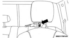
**Tether Strap Through Outboard Tether Strap Loop**
