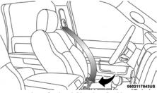
**Inserting Latch Plate Into Buckle**
