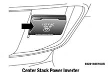
To turn on the power outlet, simply plug in the device. The outlet turns off when the device is unplugged.
