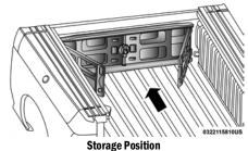
Rotate the side gates closed allowing the outboard ends to be positioned in front of the cargo tie down loops.
