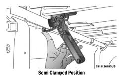
4. Push clamp handles upward to the clamped position to properly engage the clamps.
