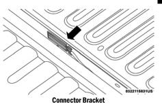
2. Remove the connector bracket from the sill by pushing inward in the locking tab.
