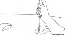
**Removing Rear Screw From Clearance Lamp**
