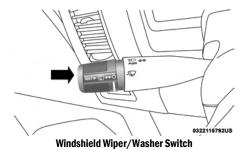
Rotate the end of the lever upward, to the first detent past the intermittent settings for low-speed wiper operation. Rotate the end of the lever upward to the second detent past the intermittent settings for high-speed wiper operation.
