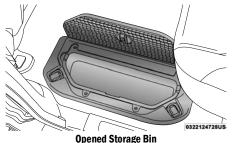
Each storage bin also contains two hooks for securing cargo. These hooks should be used to secure loads safely when the vehicle is moving.
