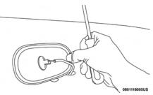
Removing Bulb Socket From Clearance Lamp
