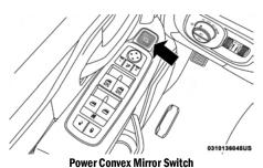
To adjust the convex portion of the outside mirrors, push the Power Convex Mirror Switch. Then, select the mirror you want to adjust by using the L (left) or R (right) buttons.
