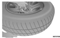
Pushing The Retainer Through The Center Of The Wheel And Positioning It
