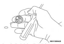
**Removing The Bulb From The Bulb Socket**
