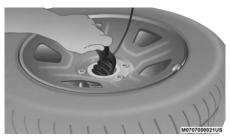
**Pulling The Retainer Through The Center Of The Wheel**
