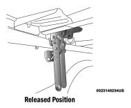
3. From the released position, send the clamps to the Stowed Position by pushing from the yellow bumper up. Listen for a "clicking" sound to confirm the clamp has been properly stowed.
