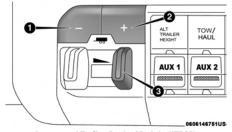
Integrated Trailer Brake Module (ITBM)
