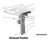
From the Released Position, send the clamps to the Stowed Position by pushing from the yellow bumper up. Listen for a "clicking" sound to confirm the clamp has been properly stowed.
