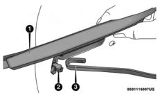
**Removing Wiper From Wiper Arm**
