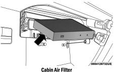
Install the cabin air filter with the arrow on the filter pointing toward the floor. When installing the filter cover, press on each end until you hear an audible click.
