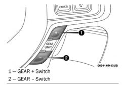
To exit ERS mode, simply push and hold the GEAR+ switch until the gear limit display disappears from the instrument cluster.
