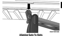
Rotate the side gates closed so that the outboard ends are secured into the intended slots of the bed.
