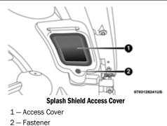
4. Reach through the access hole of the wheel house splash shield and disengage the bulb access cover by rotating counterclockwise.
