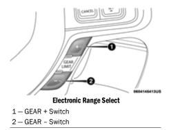
To exit ERS mode, simply push and hold the ERS (+) switch until the gear limit display disappears from the instrument cluster.
