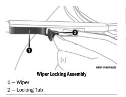
3. Tilt the lower end of the wiper blade away from the arm and use one finger push the release tab toward the wiper arm.
