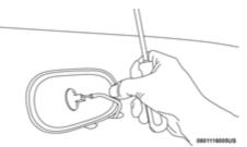
Removing Bulb Socket From Clearance Lamp
