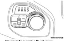
**Electronic Transmission Gear Selector**
