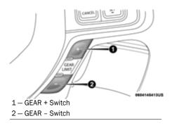
To exit ERS mode, simply push and hold the GEAR+ switch until the gear limit display disappears from the instrument cluster.
