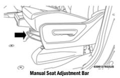
While sitting in the seat, pull up on the handle and slide the seat forward or rearward. Release the bar once you have reached the desired position. Then, using body pressure, move forward and rearward on the seat to be sure that the seat adjusters have latched.
