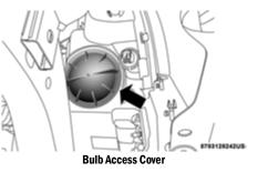
5. Disconnect the internal lamp wiring harness connector from the low beam bulb.
