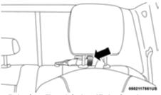
Tether Strap Through Outboard Tether Strap Loop
