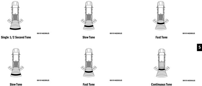
The vehicle is close to the obstacle when the warning display shows one flashing arc and sounds a continuous tone. The following chart shows the warning alert operation when the system is detecting an obstacle:
