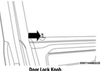
Front doors may be opened with the inside door handle without lifting the lock knob.
