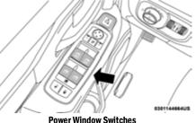
The power window controls located on the driver's door trim panel have up-down switches that give you fingertip control of all power windows. There is a single opening and closing switch on the front passenger door for passenger window control and on the rear doors for rear window control. The windows will operate when the ignition switch is turned to the ON/RUN or ACC position, and for up to 10 minutes after the ignition is turned OFF or until a front door is opened.
