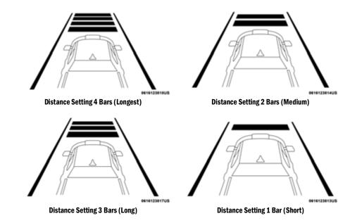
The system automatically defaults to the longest distance setting. To decrease the distance setting, push the Distance Button and release. Each time the button is pushed, the distance setting decreases by one bar. Once the shortest setting is reached, if the button is pushed again it will reset to the default setting (longest).
