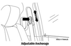
As a guide, if you are shorter than average, you will prefer the shoulder belt anchorage in a lower position, and if you are taller than average, you will prefer the shoulder belt anchorage in a higher position. After you release the anchorage button, try to move it up or down to make sure that it is locked in position.
