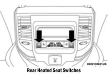
There are two heated seat switches that allow the rear passengers to operate the seats independently. You can choose from HI, MED, LO, or OFF heat settings. Amber indicator lights in each switch indicate the level of heat in use.
