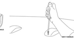
**Removing Rear Screw From Clearance Lamp**
