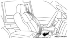
**Inserting Latch Plate Into Buckle**
