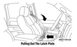
When the seat belt is long enough to fit, insert the latch plate into the buckle until you hear a "click."
