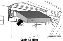
5. Remove the cabin air filter by pulling it
