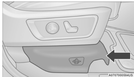
Pull Jack Access Cover From Front
