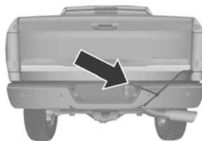
Inserting The Extension Tubes Into The Access Hole
