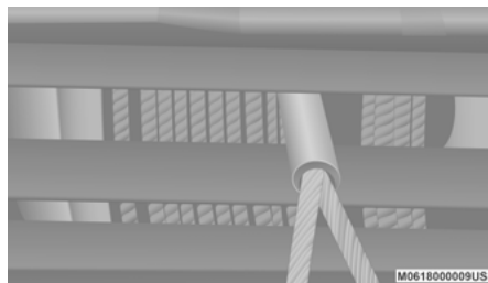
Synthetic Rope Neatly Wound Around The Spooling Drum
