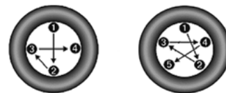
Four And Five Lug Nuts/Bolts Torque Pattern
