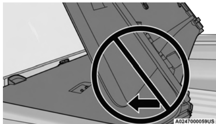
Incorrect Folding – Will Cause Damage
