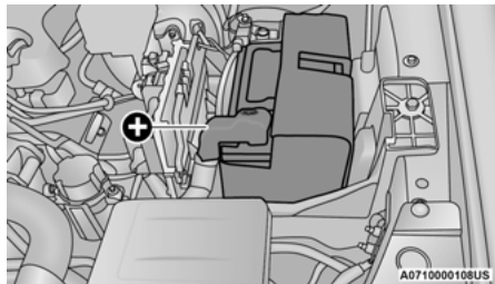
Positive (+) Battery Post
